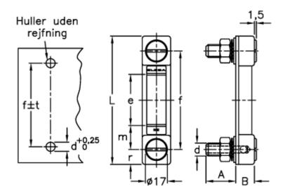
A = 23 Max tightening torque (Nm) = 12 to 15 B = 14.5 r = 11.5 C = 22 t = +/-0,5
